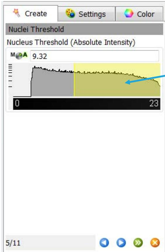
Adjust the Threshold for the grey shape to adjust to the object in the best way possible.
