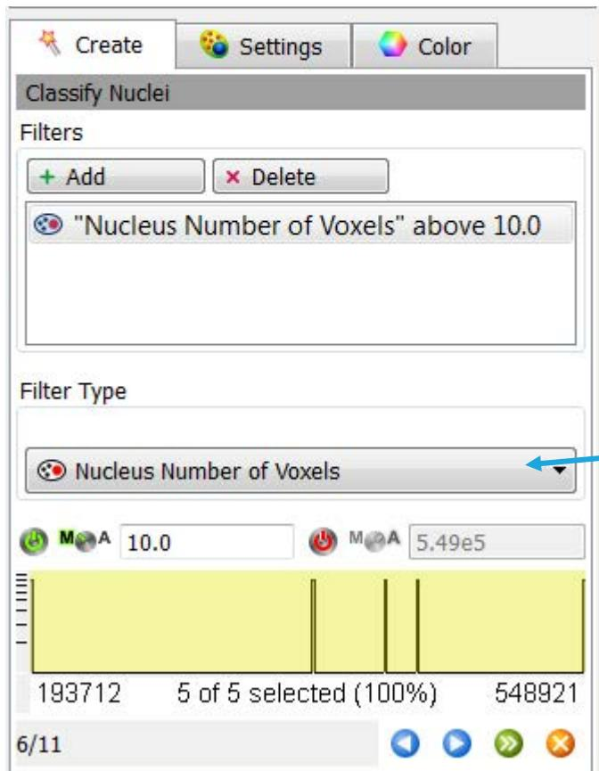
Filtering step in which you can add multiple filters in order to select the subcellular structures that are of interest.
