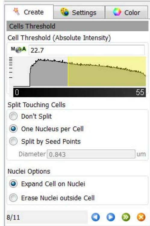
Adjust the Cell Threshold for the grey shape to adjust to the object in the best way possible.
